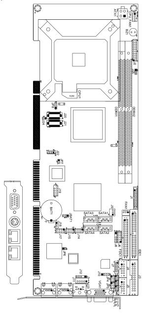
The connectors on IB940 allows you to connect external devices such as keyboard, floppy disk drives, hard disk drives, printers, etc. The following table lists the connectors on IB940 and their respective functions.
